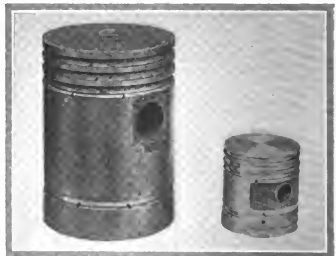
The advance in piston design made in the past five years is brought out strikingly in the two pistons illustrated above. That at the left was used in the six-cylinder Oldsmobile Limited for 1911 and 1912. It was of cast iron and weighed 6 lb., 14 oz. That at the right is the 9 oz. aluminum piston used in the new eight-cylinder Oldsmobile.
